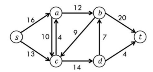
Consider the network given above with source s and sink t, with the numbers on the edges denoting maximum capacity across a particular edge. The value of the maximum flow in the given network is .
