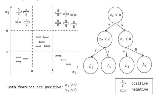
$L_1,L_2,L_3,L_4$  are leaves. The four dotted lines  $x_1=a,x_1=b,x_2=c,x_2=d$  are drawn for your reference. Both features  $x_1$  and  $x_2$  are positive. Our focus will only be on the first quadrant. Use  $\log_2$  for all entropy calculations. Calculate all intermediate quantities upto three decimal places .
